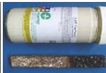
Left picture: Damaged steel bands. Right picture: CorrVerter® applied to the right side of the band; the coating has converted the corrosion into a protective layer.
