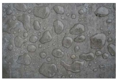
speaking, Generally the amount corrosion inhibitor is highest in pure SACI products, and lower in water-repellentbased SACIs (but these materials have the added water repellency feature that allows them to be used as a two-in-one material). Water-repellent SACIs generally have a corrosion inhibitor concentration ranging 1-10%. from depending on manufacturer, whereas a pure corrosion
