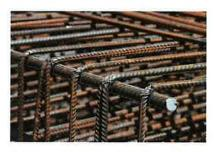
A single component, fast drying water based primer, CorrVerter® MCI® can be applied to layers of tight rust, converting it into a hydrophobic passive layer. This method reduces labor and makes rerusting less likely in the near future.
