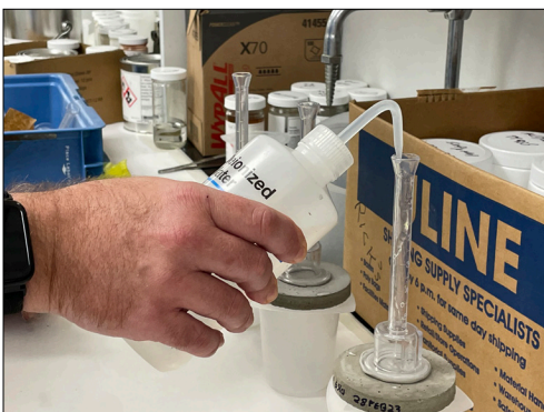
The tubes are filled with 5 inches of water, with care taken to avoid air bubbles that would interfere with water pressure in the column of water.
