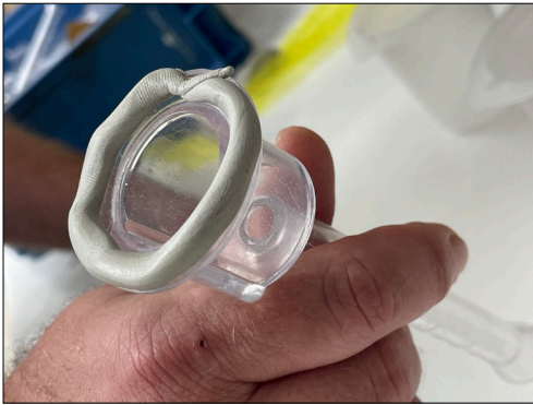
A special waterproof putty is placed on the bottom of a RILEM test tube to seal it to the concrete prior to testing.
