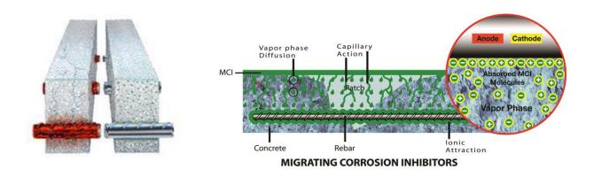
MCl<sup>®</sup>2020 is recommended for: preventative maintenance of existing reinforced, precast, prestressed, post-tensioned, or marine concrete structures , bridges, highways, and industrial
