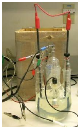
Figure 5 – Test setup of ASTM G180
