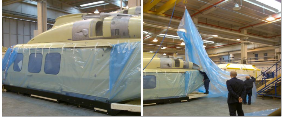
Corrosion protection of an “AW 139” helicopter fuselage to be ocean shipped to Baltimore, USA. Solution: VpCI®-126 film integrated with VpCI®-137 foam.
