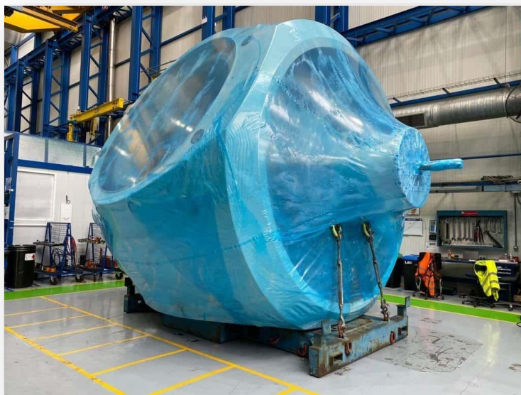
Powerfull VpCI®-126 HP UV Shrink Film provides strong multi-metal protection for parts and equipment.
