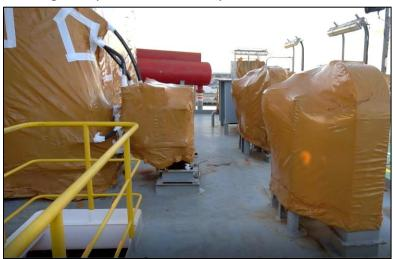
Equipment wrapped in MilCorr® VpCl® Shrink Film has been proven to survive hurricanes. Several aircraft cargo loaders underwent testing to evaluate the performance of a VpCl® preservation system for extending asset life expectancy. After a variety of VpCl® materials were applied internally, the assets were wrapped in MilCorr® VpCl® Shrink Film and stored outside. Three hurricanes hit the whole
