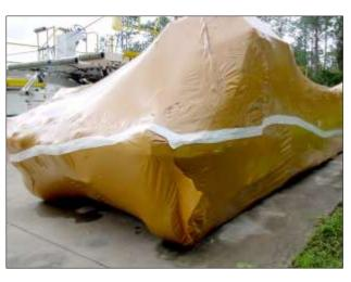
In many of these cases, MilCorr<sup>®</sup> is the finishing touch for a full-fledged preservation of the system. Depending on the asset being preserved, other layup steps may include the prior addition of VpCI<sup>®</sup> Additives to oil systems, VpCI<sup>®</sup> Coatings to bare metal surfaces, VpCI<sup>®</sup> Emitters to electrical compartments, and VpCI<sup>®</sup> Pouches, Foams, or Fogging Fluid where additional VpCI<sup>®</sup> is needed to protect large internal volumes.
