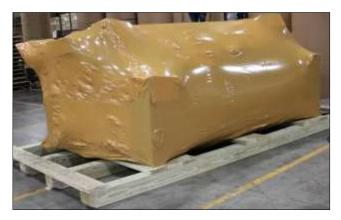
In addition to serving as both an excellent physical barrier and corrosion inhibitor, MilCorr® VpCI® Shrink Film is extremely easy to use. It can eliminate the need for conventional rust preventatives such as oils and greases that require a messy cleaning process before the equipment can be put back into service. MilCorr® offers the advantage of corrosion protection with no cleaning or degreasing required, so equipment is basically ready
