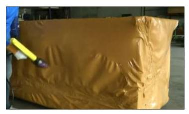
Once any internal asset preservation steps have been taken care of, MilCorr® VpCI® Shrink Film should be cut to the desired size with enough excess for overlap at the seams. The next step is to lay out the MilCorr® in a clean dry area, place the vehicle or equipment on the VCI film, pad off any sharp edges and corners (this is especially important to prevent holes in the film where the
