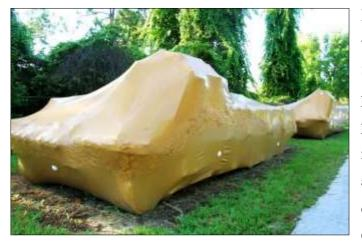
In addition to the durable barrier it provides against the elements, the key advantage of MilCorr® VpCI® Shrink Film is its ability to replace conventional rust preventatives such as oils and desiccants. Parts protected with MilCorr® VpCI® Shrink Film are ready to use immediately after removal, saving time and money by eliminating the need for additional cleaning or degreasing. In conjunction with other Cortec® products, MilCorr® VpCI® Shrink Film
