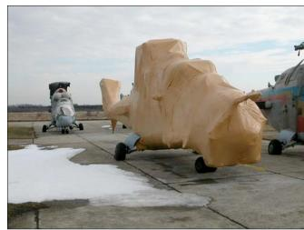
Cortec® MilCorr® VpCI® shrink films conform to military specification MIL-B-22019D, NACE Standards RP0487-2000, and TMO-2008.
