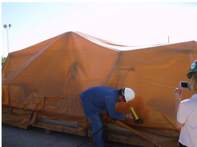
Shrink-wrapping of the film with the heat gun.
