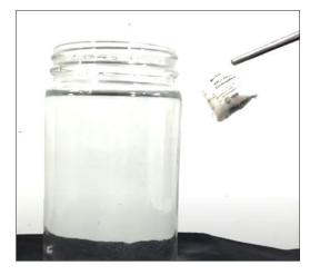
We are pleased to present a new demo video on MCI<sup>®</sup>\_Mini Grenades! For 20 years and counting, MCI<sup>®</sup> admixture has been available packaged in small water-soluble bags for ease of use and convenience. These MCI<sup>®</sup> Grenades can be added to concrete, repair mortar, and grout mixing water for enhanced corrosion protection. Our new video shows an up-close look at what happens when these pre-dosed pouches come in contact with mix water!
