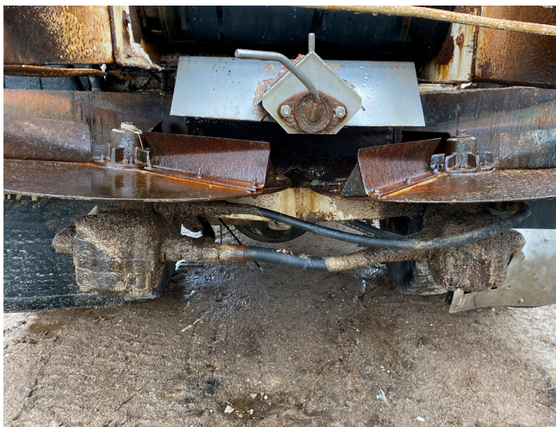
Figure 1. The impact of corrosion on a fertilizer spreader truck. Image courtesy of Cortec®/Anthony Price.
