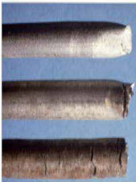
Figure 29: Collapse of suspended ceilings in swimming halls due to inappropriate stainless steel fastening elements. Failure by stress corrosion cracking. 41
