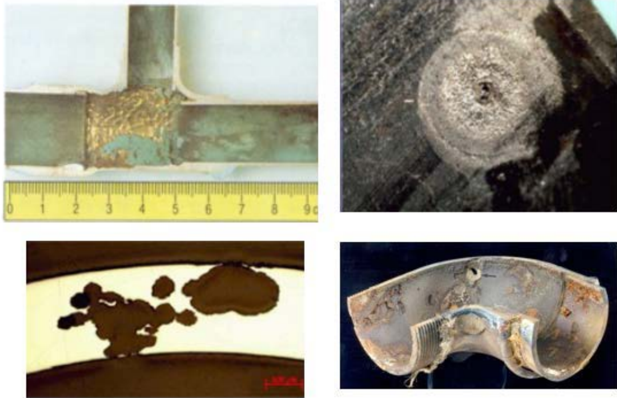
Figure 8: Corrosion failures in plumbing systems. Clockwise from top left: Erosion-corrosion of copper piping, pitting of stainless steel by chlorine disinfection (surface view), pitting of stainless steel by chlorine disinfection (cross section through pipe wall), and pitting of galvanized steel piping.
