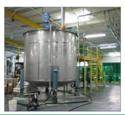
The addition of a new 5,000 gallon (18,927 L) liquid blending line earlier this year signals continued growth at the Cortec® Biotechnology Campus (CBC) in Sarasota, Florida. With 4500 workable gallons (17,034 L), the line is able to produce twice as much product in one batch as it was previously able to make in smaller tanks at CBC.
