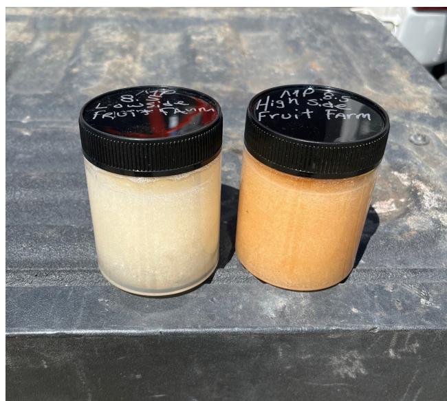
Figure 4. CorroLogic VpCI Gel is pumped through the filler pipe into the lower portion of the casing until it can be detected coming out the other side. Inevitably, it often picks up some of the debris contaminating the inside of the casing, which is why the right sample is darker than the left one. (Source: Cortec, courtesy of Eric Uutala)
