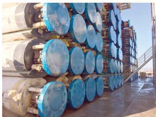
Figure 1: Hot layup of risers on a drillship using waterborne VCI fogging and capping with film. All images courtesy: Cortec Corp.
