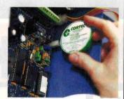
VpCI-105 emitters emit Vapour phase Corrosion Inhibitors (VpCIs), which form a monomolecular protective coating on all metal surfaces.
