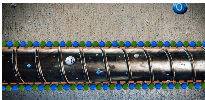
Figure 1. Illustration of MCI molecules adsorbing on and protecting rebar against corrosive elements that make their way through the concrete pore structure.
