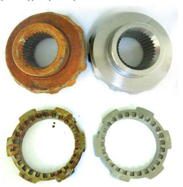
When Cortec® Laboratories subjected a variety of sintered metal gears, locking plates, and pinions to ASTM D-1735 humidity testing at its IEC 17025 accredited lab, it saw a marked difference between parts
