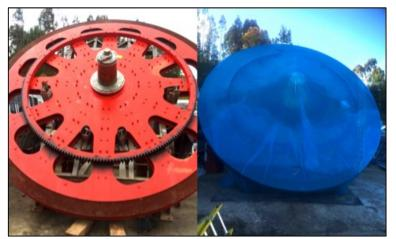
Cortec® has integrated Vapor phase Corrosion Inhibitor Technology into a variety of different packaging materials to provide flexible and effective protection solutions for metal parts and equipment of all sizes. For the outside of equipment or parts, VpCI® film such as MilCorr® and VpCI®-126 HPUV combine corrosion protection with high durability characteristics to withstand the
