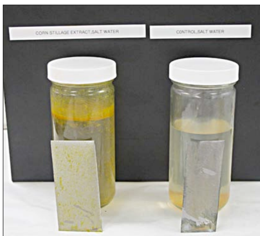
Above: Panel removed from the solution containing corn stillage extract. This panel is covered with the thick film which basically acts as an air / moisture / salt barrier. This film is easily removed using VpCI®-418LM (non-foamy detergent).
