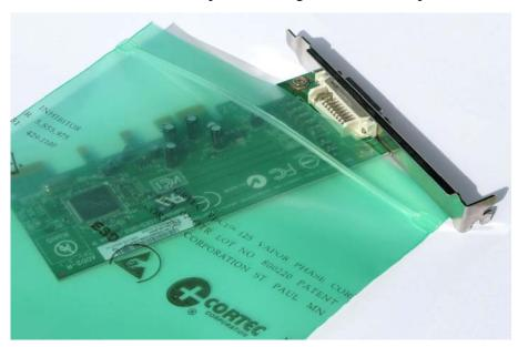
VpCI<sup>®</sup>-125 is used by world leading electronic companies like Nortel Networks and Motorola Inc. Motorola wanted cost effective and less time consuming method of export packaging. VpCI<sup>®</sup>-125 antistatic bags were selected and placed over the enclosures resulting in better protection and reduction of packaging material and labor.
