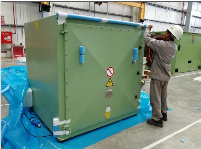
After sharp-edge protection terminal boxes were packed and heat shrunk in VpCI®-126 HP UV Shrink Film for external preservation.
