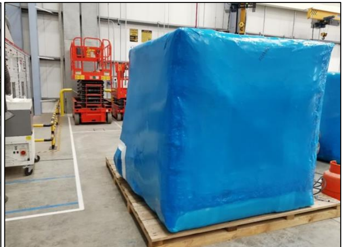
After sharp-edge protection terminal boxes were packed and heat shrunk in VpCI®-126 HP UV Shrink Film for external preservation.
