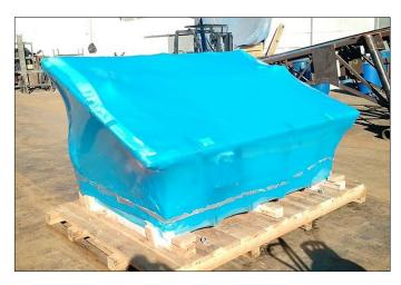
Inhibitors that form a protective layer on the external equipment surface. Packaging such as this is superior
