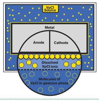
Vapor corrosion inhibitor technology releases vapors that disperse throughout the equipment to be protected and fill void spaces. The corrosion protection materials form a protective molecular layer on metal surfaces inside the enclosure.
