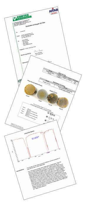
Not all brands of VCI (Vapor Corrosion Inhibitor) film are equal, as Cortec<sup>®</sup> has found testing a variety of products, including a 3-mil sample of Propak VCI film near the end of 2018. The film sample (received in 2017 in good condition) recently underwent testing according to Razor Blade Test (Cortec<sup>®</sup> test method CC-004) and NACE Standard VIA (Vapor Inhibiting Ability) Test (NACE TM0208-2008).\* These tests evaluate two different aspects of corrosion protection:
