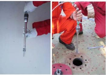
Figure 6: Weight Loss Corrosion Coupons
