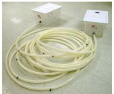
Figure 1: Testing apparatus for verifying VCI diffusion with no air movement
