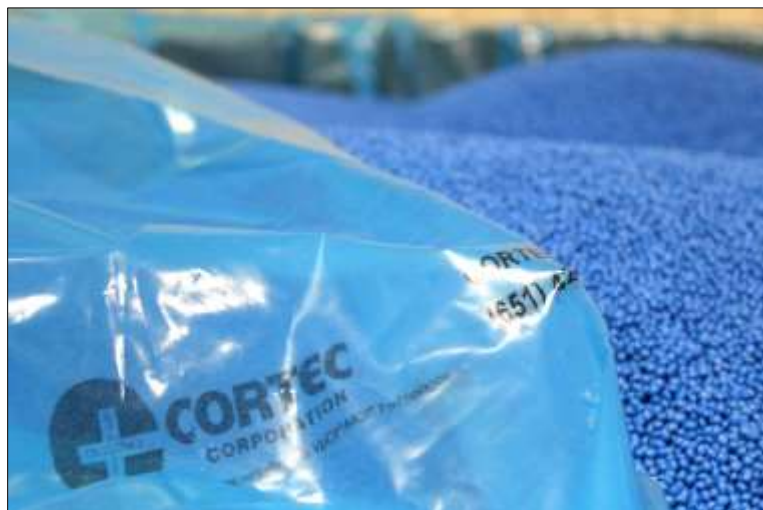
VpCI® Films and Bags Recycled into Reprocessed Resins for Use in Extrusion and Converting Downstream.
