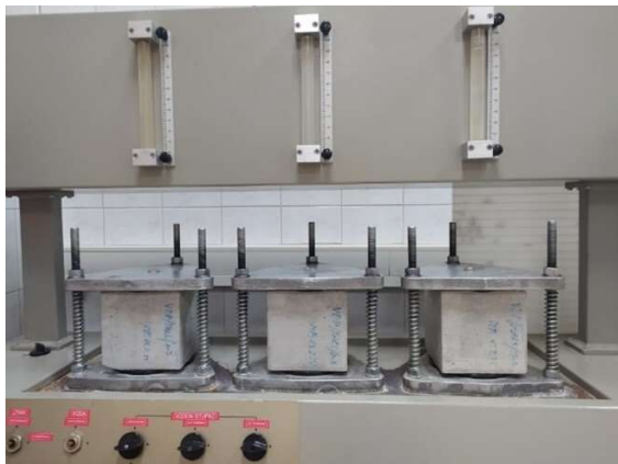
Figure 6 Device for testing the depth of water penetration under pressure and the limit value of the maximum water penetration for different classes according to HRN 1128:2007
