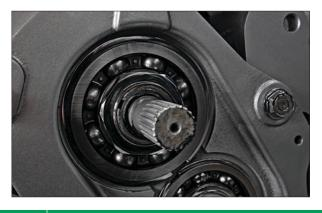
Once the bearing is restored, allow it to dry before reinstalling it with the appropriate lubricant. If the bearing needs to be laid up for later use, choose from a wide array of VpCI® packaging materials (VpCI® Paper, Films, Foams) for dry corrosion protection without any special coatings application or removal required.
