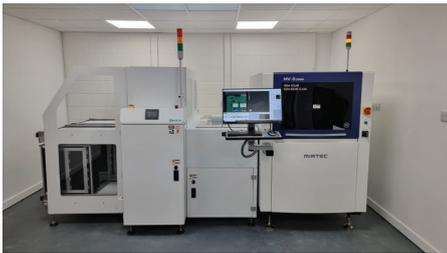
The AOI system is the multi award-winning Mirtec MV-6 Omni 3D Inspection system, which is recognised as having the best cameras, 3D sensors, Z-axis and double-sided inspection capability available, as well as a lighting array combined with automatic programming and debug software to provide unparalleled inspection quality.
