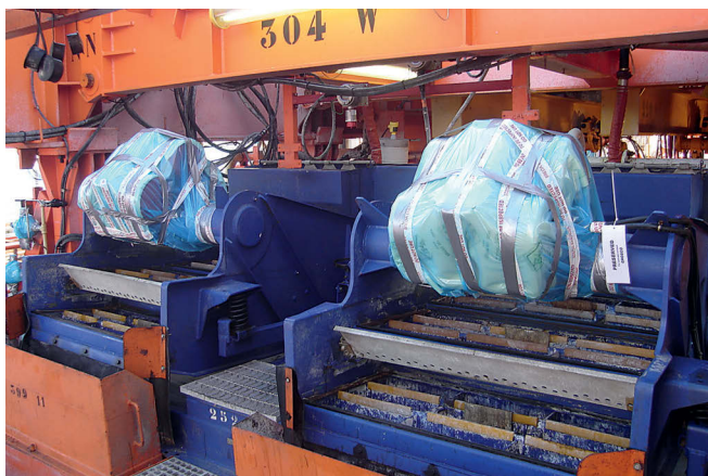
DC Motors on a mud pump were protected with VpCI foam and film during temporary lay-up on an offshore rig in the Mediterranean (source: Cortec Case History 303)
