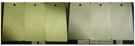
PTC Emitters diffuse 30m (100 ft) in a closed space without air movement and provide corrosion protection at the distance of 30 m from the source of MCI  $^{\circledR}$
