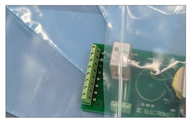
One of the core packaging solutions for protecting sensitive electronics is Cortec's line of EcoSonic<sup>®</sup> VpCI<sup>®</sup>-125 Static Dissipative Film & Bags. As their name suggests, these bags combine the best multi-metal corrosion protection with strong static dissipative properties. They contain Vapor phase Corrosion Inhibitors to protect void spaces and recessed areas within the package—no coating
