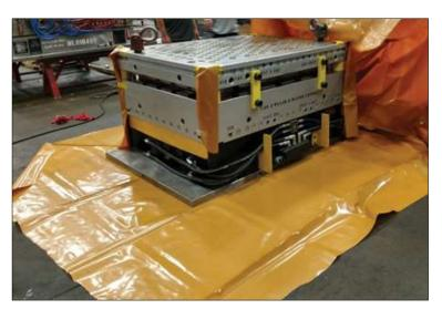
One common challenge for molders is finding a place to store large high-dollar equipment between jobs. Too often, expensive molding equipment ends up outdoors, subject to corrosive conditions that require rust removal by the time the mold is brought back indoors for use. In these situations, EcoAir<sup>®</sup> 325 Tool & Die Rust Preventative can be supplemented by adding a VpCI<sup>®</sup>-309 Pouch inside the mold cavity and wrapping the entire piece of tooling
