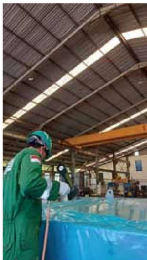
➤ Shrink wrapping heat exchanger with corrosion inhibiting film. Image courtesy of Tiga Ombak, Cortec® Case History 852.
