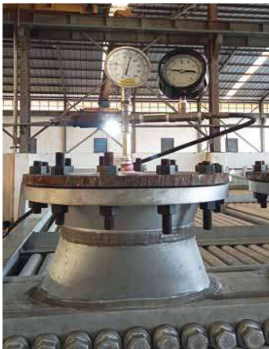
➤ Closeup of pressure gauges for hydrotesting of heat exchangers. Image courtesy of Tiga Ombak, Cortec® Case History 852.
