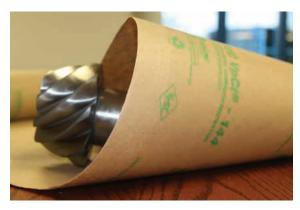
very advantageous over oily rust preventatives because they create less mess and minimise or eliminate the hassle of rust preventative removal and disposal.
