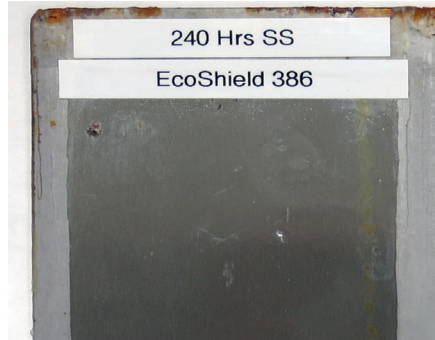
EcoShield 386 coating protection from corrosion compared to a conventional DTM coating.
