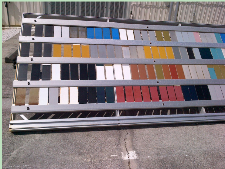
ASTM exposure rack for testing weathering resistance of VpCI® coatings. The rack is located at Cortec® Biotechnology Campus in Sarasota, Florida, in a semitropical climate in the vicinity of the Gulf of Mexico.
