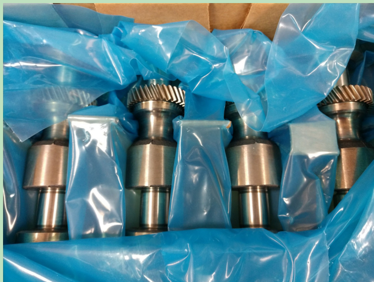
Bulk-wrapped parts with no observed corrosion after 72 hours of testing in ASTM 1735 conditions.
