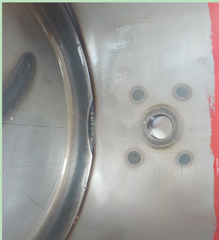
Tank section after 96 hours of testing in ASTM B117 salt spray conditions.
