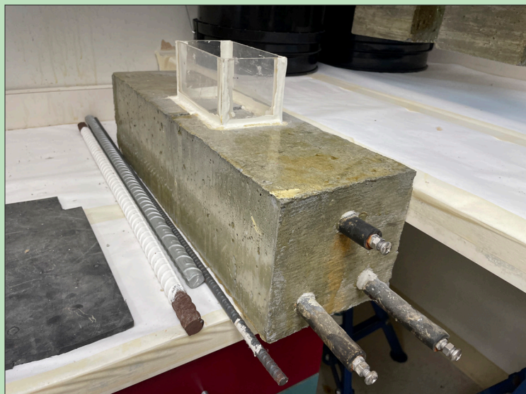
Standard setup for ASTM G109: container on top for saltwater ponding, upper rebar located nearer the surface for exposure to saltwater, lower two rebars protected from saltwater by thick concrete cover. The upper and lower rebars are connected with a wire to measure the difference in corrosion potential and calculate the corrosion rate.
