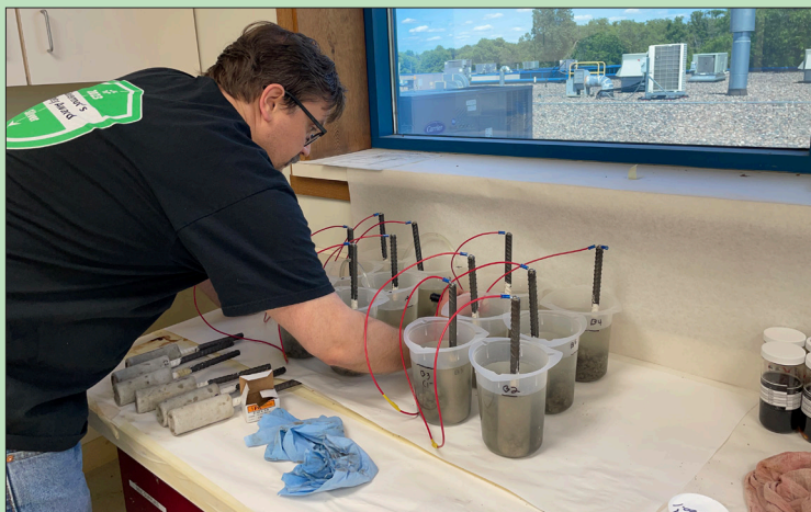
Colin setting up "lollipop" samples for "rapid microcell corrosion testing" with slight modifications to improve upon the process previously explored by the Texas DOT.
