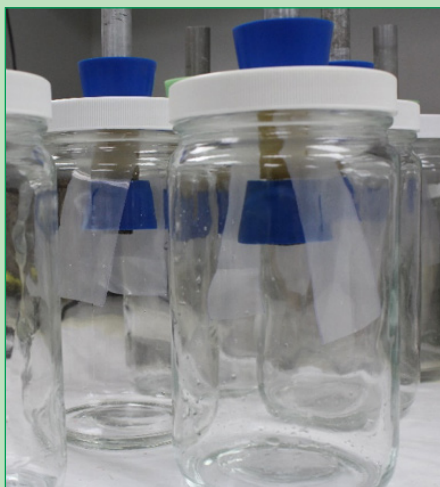
NACE TM 0208-2018 VIA testing in action
