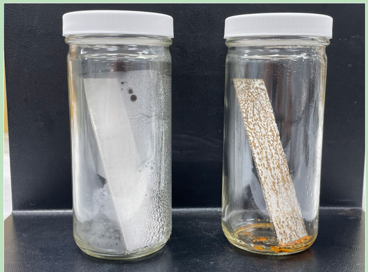
Variation on ASTM G31 Immersion Testing. These jars simulate hydrotesting conditions. The panel at left was treated with a 0.3% solution of VpCI®-649 BD. The panel at right was untreated in DI water and shows signs of corrosion.
