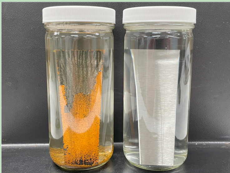
ASTM G31 Immersion Testing. After approximately 10 days in immersion testing in a 104 °F (40 °C) oven, the control panel (left) shows corrosion while the panel in a 0.3% solution of VpCI®-649 BD (right) is still bright, corrosion-free metal.
