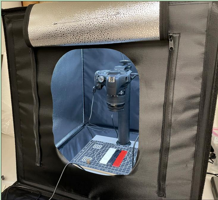
The new DSLR camera mounted at a specific angle with uniform lighting will improve the quality of pictures, making it easier for the computer software to detect areas of rust vs. non-rust.
