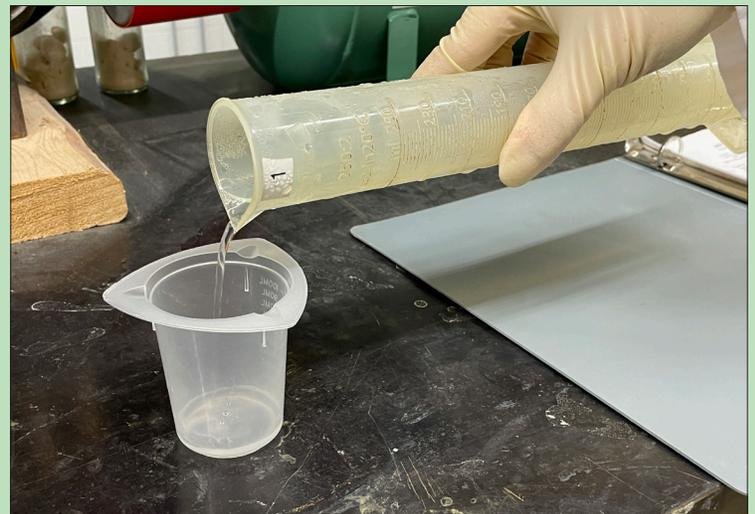
*Our Lab Tech combines the water collected in the two cylinders to test pH on a regular basis.*
