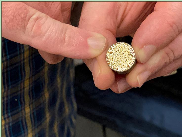
*Colin points out rust spots on a steel plug used for VIA testing. The NACE VIA test uses a grading method based on the relative number of corrosion spots to evaluate whether a corrosion inhibitor passes or fails the test. Colin believes that he will be able to measure the amount of corrosion more precisely with computer software.*
