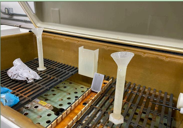
*The Q-Fog chamber houses two graduated cylinders that collect water droplets in the humidity chamber. This allows our Lab Tech to measure how much fog is accumulating per hour and make sure it stays within the range of ASTM 1735 specs.*
