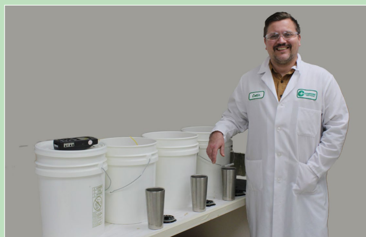
Colin has created four calorimeters to measure set time. He can test up to four samples per day.
