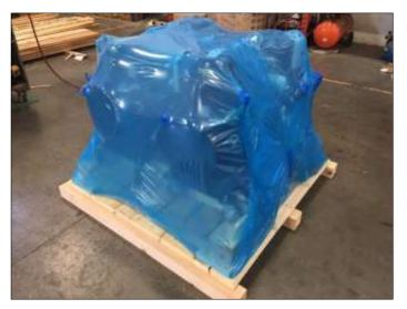
The risk for corrosion is especially high in non-climate-controlled warehouses or shipping containers that experience extreme temperature and humidity swings or are located in seaside environments. Longtime assets or newly manufactured goods can gradually rust and deteriorate if not sufficiently protected, leading
