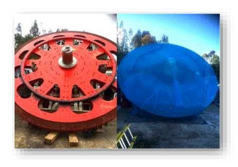
protection for and parts equipment for up to three years in aggressive outdoor conditions. Unlike some preservation films that rely on white pigments to reflect UV light, VpCI®-126 HP UV contains unique inhibitors that protect the polymer from UV exposure and prevent degradation. VpCI®-126 HP UV is translucent and can be applied in numerous applications. It is ideally suited for transit staging and layup of critical equipment; including equipment with large void spaces,
