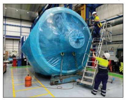
components were shipped out along with VpCl®-414 as part of a complete kit to clean off VpCl®-368 D at the destinations when required. After testing Cortec® VpCl® materials, the customer ultimately decided to incorporate them into their new wind turbine projects to avoid corrosion problems from the past and commented on how easy the system was to apply.
