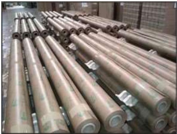
Cortec® came to the rescue by providing VpCI®-148 Paper. Cortec® was the only supplier able to produce the rolls of grease resistant paper at almost 2.5 meters (98") wide, the size needed to wrap the large frames. VpCI®-148 Paper eliminated the tarnish and corrosion problem even in the presence of process oil, thus proving to be more suitable for the application than the previously used VCI polyethylene film.
